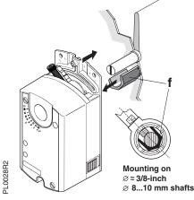
Remove factory installed 1/2-inch guide. See Figure 4.
